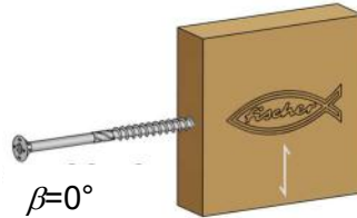
Figure D6.1: Screw arrangement in the narrow surface of WBP (figure not to scale)
